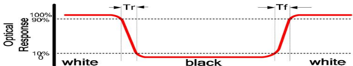
FIG2. Measuring method for Contrast ratio,surface luminance,Luminance
