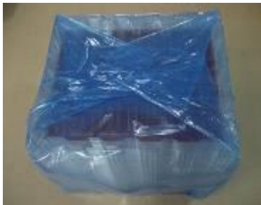
7 - Insert the package from the sideway of the Antistatic Bag. Pack the bag, and then tape with scotch tape.
