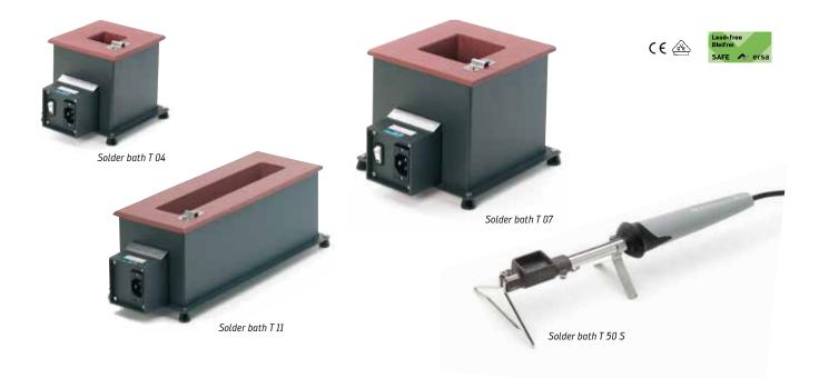
Ersa solder baths are electrically heated melting pots for solders. The high-capacity ceramic heating elements are exchangeable and mounted on the pot. They are thermally insulated from the external sheet metal housing.
