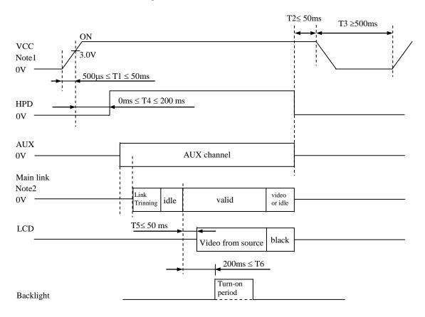
Note1: If there is a voltage variation (voltage drop) at the rising edge of VCC below 3.0V, there is a possibility that a product does not work due to a protection circuit.
