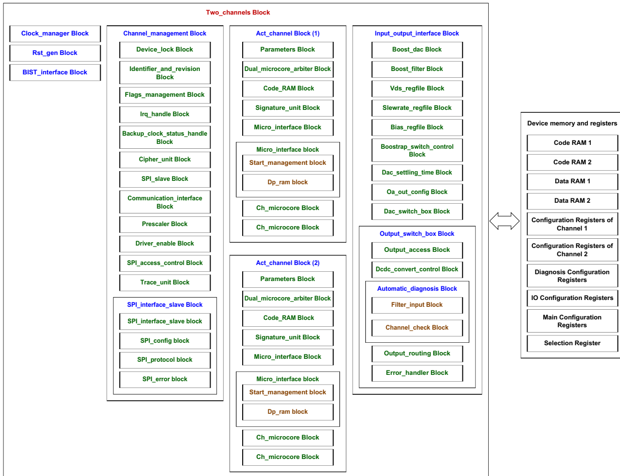
Figure 24. Device logic block hierarchic overview
