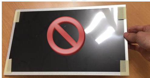
Do not lift and hold the panel with Single hand at right or left side from tray.
